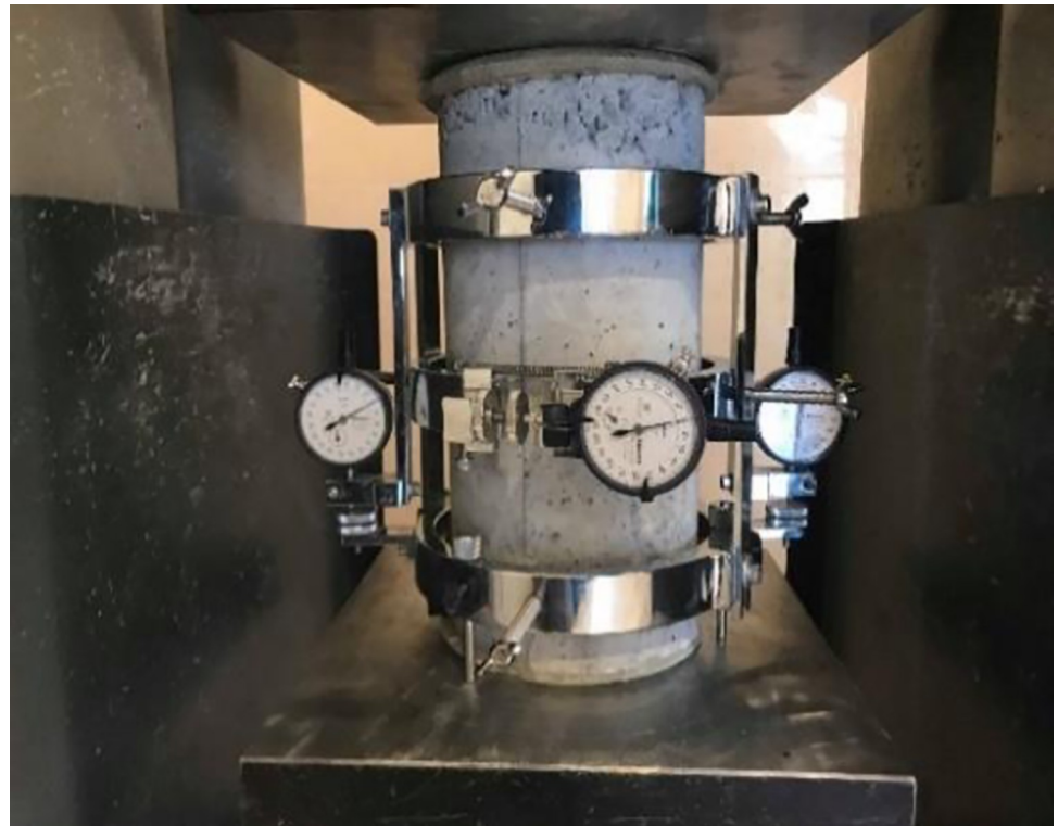
Fig 2. Modulus of elasticity test using compressometer.
