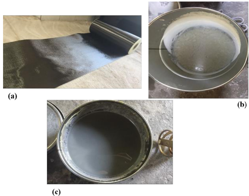
Fig 4. CFRP and epoxy resin: (a) CFRP roller; (b) epoxy resin component A; and (c) epoxy resin component B.
