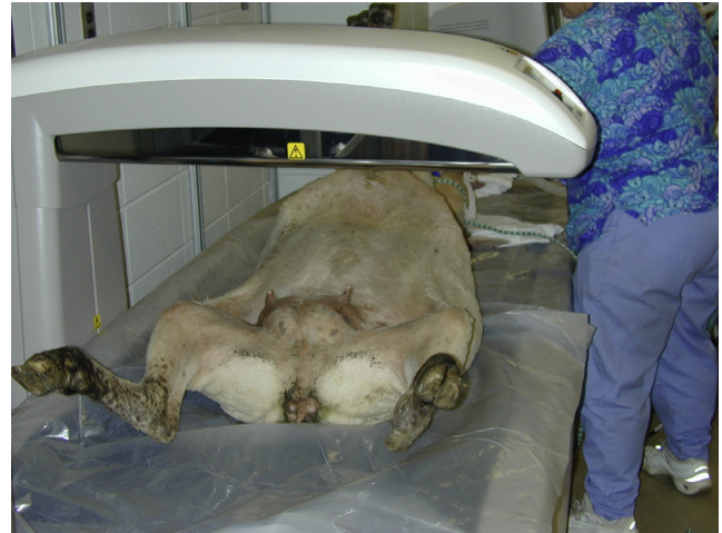
Fig. 1. DEXA scan of the lumbar spine (L3-L6) using GE Lunar Prodigy DPX X-Ray bone densitometer Scanning procedure with anaesthetized sheep positioned in ventro-dorsal recumbency.
