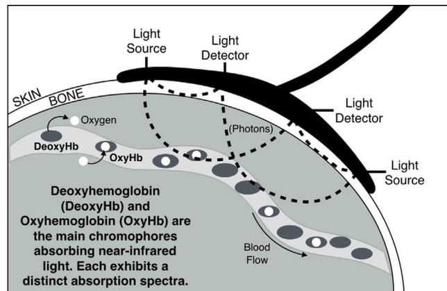
**Fig. 3 – The use of NIRS to determine cerebral regional cerebral oxygen (rSO<sub>2</sub>) saturation. Using algorithms, the cerebral oximeter subtracts oxygenation in bone, skin and dura (dark dashed curved line) and determines balance between cerebral oxy/deoxyhemoglobin.**
