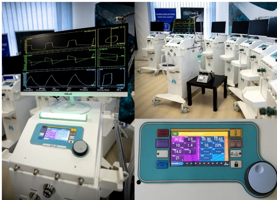
Fig. 1. Luca mechanical ventilator with close-up of the user interface (online version: colour; print version: black and white).
