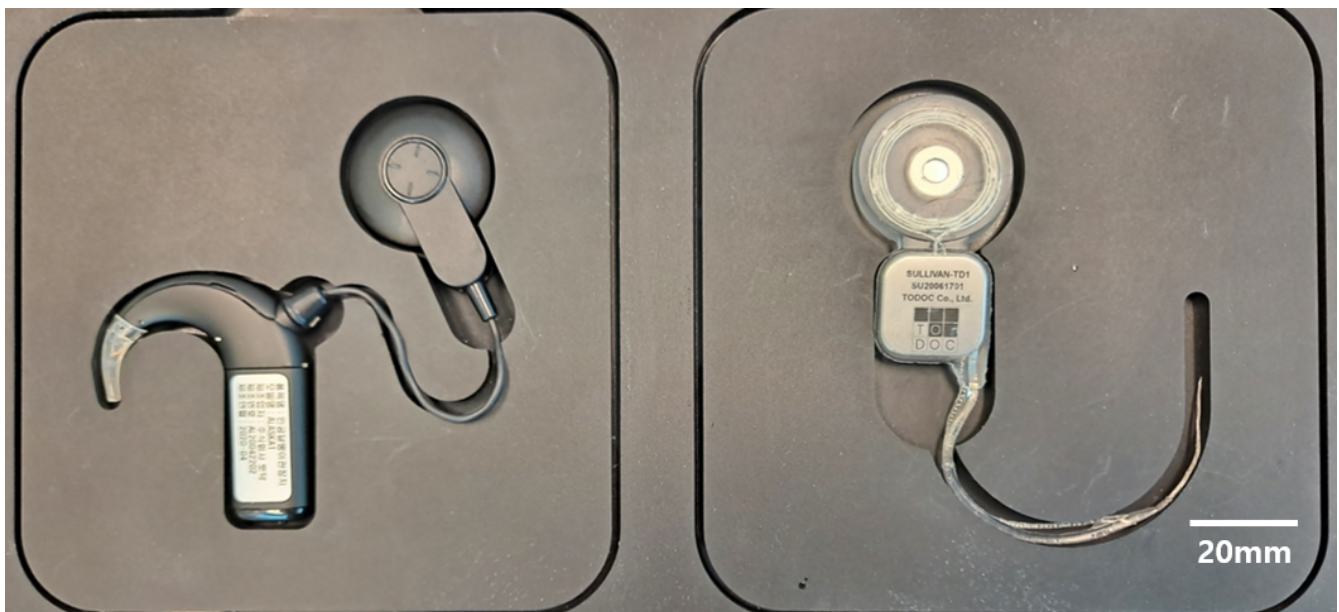
Figure 10. TODOC's 32-Channel Cochlear Implant Sound Processor (Left) and Implantable Pulse Generator (Right). The 32-channel cochlear implant system consists of 32-channel neural stimulation and recording IC, titanium-based hermetic package, and sound processor with wireless power and signal transmission coil.
