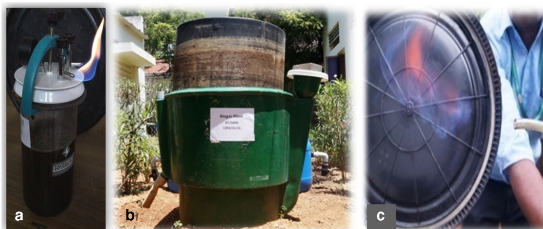
Fig. 6. Flame test with the methanation plants. (a) Lab-scale bench-top methanation unit. (b) Pilot-scale bio-methanation plant and (c) flame test.
