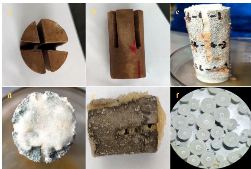
Figure 8. Experimental results of phase change in complex fractures under formation conditions. (a,b) Core cutting to simulate complex fractures. (c–e) Solid particles completely fill in fractures. (f) Microstructure of solid particles cured in complex fractures.
