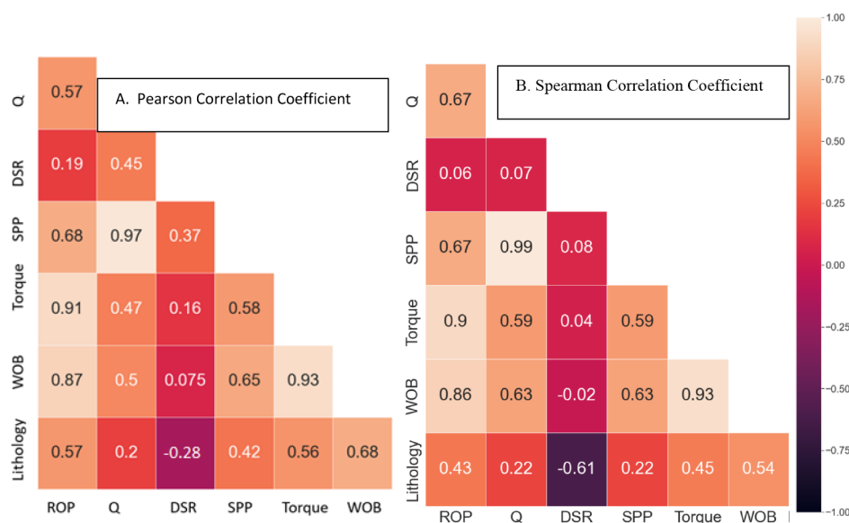
Figure 3. Correlation coefficient of the parameters with formation tops: (A) Pearson correlation coefficient. (B) Spearman correlation coefficient.
