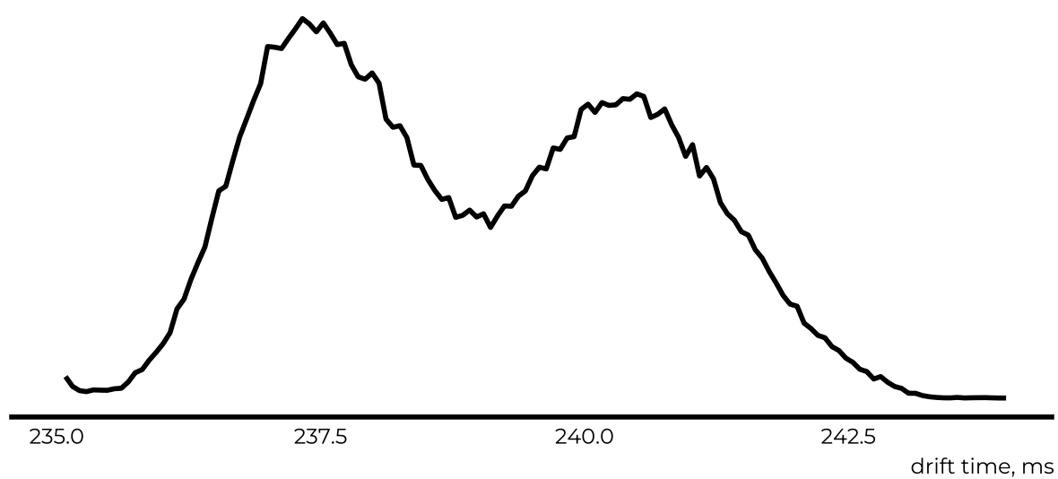
Figure S9 High resolution ion mobility separation (29 cycles) of monuron and 3-(3-chlorophenyl)-1,1-dimethylurea.
