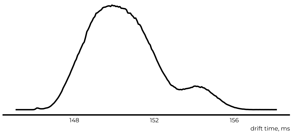
Figure S7 High resolution ion mobility separation (14 cycles) of sebuthylazine and terbuthylazine.
