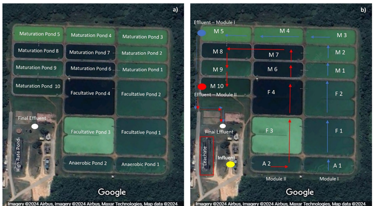
Fig. 1. View of the Belém Novo WWTP (a) Identification of the modules, (b) identification of the effluent flow represented by the arrows: in red, module II that receives the leachate and, in blue, module I that does not receive the leachate. A, anaerobic pond; F, facultative pond; M, maturation pond.
