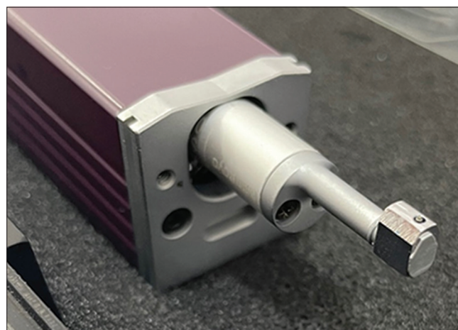
Figure 2: The diamond tip of the stylus profilometer
