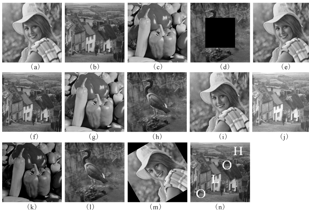
Figure 5. The attacked watermarked images. (a) Gaussian low-pass filtering (PSNR = 32.54); (b) average filtering (PSNR = 32.42); (c) median filtering (PSNR = 34.9); (d) occlusion (PSNR = 15.06); (e) JPEG (PSNR = 35.95); (f) unsharp (PSNR = 27.74); (g) blurring (PSNR = 34.03); (h) Gaussian noise (PSNR = 32.89); (i) salt & pepper noise (PSNR = 28.5); (j) brighten (PSNR = 14.15); (k) darken (PSNR = 14.52); (l) rescaling (PSNR = 34.67); (m) rotation (PSNR = 13.17); (n) painting (PSNR = 20.34).
