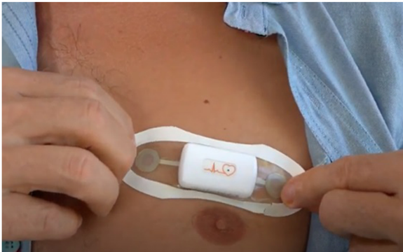
FIGURE 1 Medical devices and technical specifications used for Remote Patient Monitoring (A) Health Monitor DakikApp: blood pressure, heart rate, O_2 -saturation, blood glucose; (B) Holter ECG DakikApp: 24 h Holter ECG (One Channel), live ECG, heart rate variability, telemetry)
