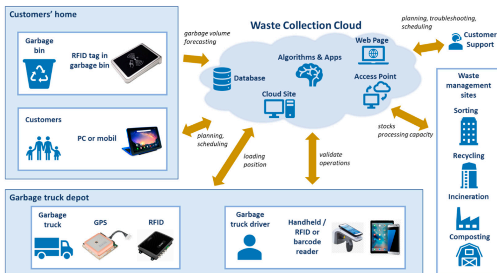
Figure 9. The Waste Collection Cloud and its connections with the cyber-physical waste collection system including customers, garbage trucks, waste management sites and customer support.
