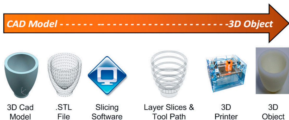
Figure 1. The 3D printing process (adapted with permission from reference [18]).
