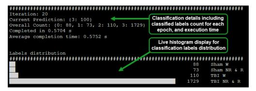
Figure 3. Live classification display for the RPi based system (64 s epoch, batch size: 100).
