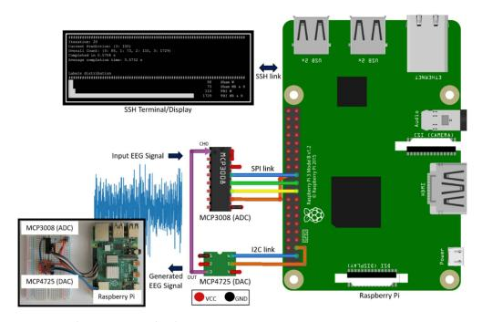
Figure 1. Deployment system hardware setup.
