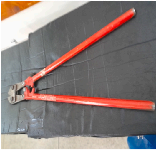
Fig. 5. Industrial Manual Scissor Metal cutter(IMSMC) which was used to remove the nut.
