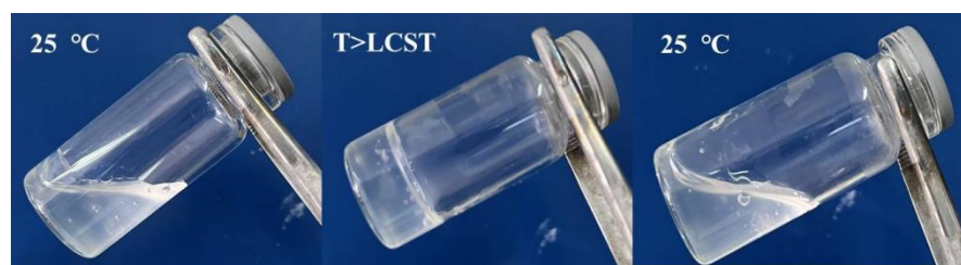
Figure 1. Digital photos of samples at room temperature (25 °C), at or above gelling temperature ( T > LCST ), and at room temperature (25 °C) (In the example, the thermosensitive gel was composed of poloxamer407, poloxamer 188, and carbomer).
