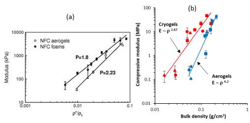
**Figure 6.** Compressive modulus as a function of (**a**) relative density for aerogels and foams based on CNF [85] (Reprinted from Composites Science and Technology, 71, Sehaqui, H.; Zhou, Q.; Berglund, L.A. High-porosity aerogels of high specific surface area prepared from nanofibrillated cellulose (NFC), 1593–1599, Copyright 2011, with permission from Elsevier) and (**b**) as a function of bulk density for aerogels and cryogels (or foams) based on cellulose II [89].
