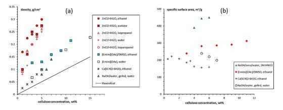
**Figure 7.** (a) Density (data are from the references: [40,121–124]) and (b) specific surface area (data from references [40,122,125,126]) of cellulose II aerogels as a function of cellulose concentration in solution, all for the dissolved microcrystalline cellulose or dissolving pulp in different solvents (first position in the legend) and coagulated in different non-solvents (second position in the legend); the solid line in (a) corresponds to the case of no shrinkage.
