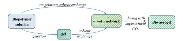
Figure 1. Schematic presentation of bio-aerogel preparation.
