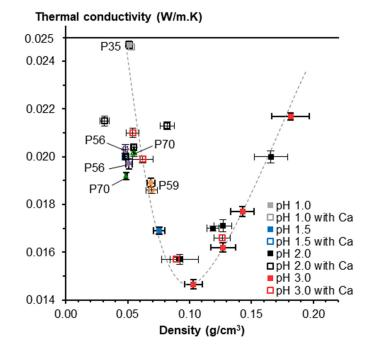
**Figure 28.** Thermal conductivity of LM pectin [16]. Reprinted from Carbohydrate Polymers, 196, Groult, S.; Budtova, T., Thermal conductivity/structure correlations in thermal super-insulating pectin aerogels, 73–81, Copyright 2018, with permission from Elsevier.
