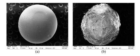
**Figure 15.** SEM surface morphology of alginate particle: (**a**) after scCO<sub>2</sub> drying and; (**b**) after resveratrol loading [242]. Reprinted from The Journal of Supercritical Fluids, 163, dos Santos, P.; Viganó, J.; de Figueiredo Furtado, G.; Cunha, R. L.; Hubinger, M. D.; Rezende, C. A.; Martínez, J., Production of resveratrol loaded alginate aerogel: Characterization, mathematical modeling, and study of impregnation, 104882, Copyright 2020, with permission from Elsevier.
