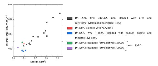
**Figure 24.** Evolution of the thermal conductivity as a function of density. Ref A: [273], Ref B: [277], Ref C: [278], Ref D: [280]. The shape of the symbol represents the drying method: square for ambient drying, circle for drying at 65 °C and triangle for drying under scCO<sub>2</sub>.
