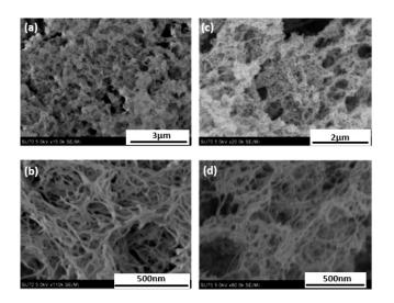
**Figure 33.** SEM images of an unloaded silk fibroin aerogel (**a**,**c**) and aerogel loaded with ~21 wt% ibuprofen (**b**,**d**). Each set of images are for the same sample at two different magnifications [390]. Reprinted from The Journal of Supercritical Fluids, Michael A. Marin, Rajendar R. Mallepally, Mark A. McHugh, Silk fibroin aerogels for drug delivery applications, 84–89, Copyright 2014, with permission from Elsevier.
