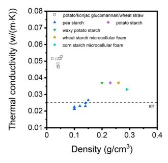
**Figure 32.** Thermal conductivity of various monolithic porous starch-based materials obtained via supercritical CO<sub>2</sub> drying (filled points) and freeze drying (open points) [36,364,372].
