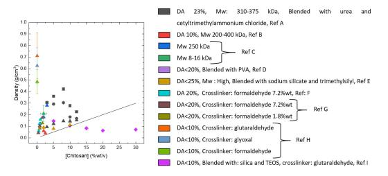
**Figure 20.** Variation of the density as a function of the chitosan concentration. Methods of drying are represented by squares for ambient drying, circles for drying at 65 °C, diamonds for freeze drying and triangles for supercritical drying. The solid line represents the density for pure chitosan materials without shrinkage and without mass loss. Ref A: [273], Ref B: [274,275], Ref C: [276], Ref D: [277], Ref E: [278], Ref F: [279], Ref G: [280], Ref H: [281], Ref I: [282].
