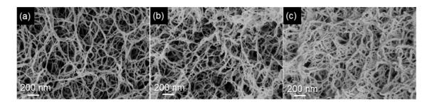
**Figure 27.** SEM images of LM pectin aerogels from 2 (**a**), 4 (**b**) and 6 wt% (**c**) solutions at pH 2 cross-linked with calcium [16]. Reprinted from Carbohydrate Polymers, 196, Groult, S.; Budtova, T., Thermal conductivity/structure correlations in thermal super-insulating pectin aerogels, 73–81, Copyright 2018, with permission from Elsevier.
