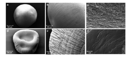
**Figure 14.** SEM images of: (**a**) alginate aerogel spherical beads after scCO<sub>2</sub> drying; (**b**) magnification of surface; (**c**) and internal porous network; (**d**) collapsed structure of alginate bead after freeze-drying; (**e**) magnification of surface; (**f**) and internal structure. Reprinted from [232].
