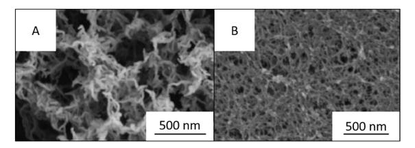
**Figure 21.** Morphology of chitosan aerogels (**A**) 2.5 w/v% chitosan, DA = 10%, MW 200–400 kDa, solvent 2%v acetic acid [275], and (**B**) 0.4 wt/v% chitosan, DA < 20%, solvent 2%v acetic acid, crosslinker formaldehyde 7.2 wt% [280]. (adapted with permission from Takeshita, S.; Yoda, S. Chitosan aerogels: transparent, flexible thermal insulators. Chemistry of Materials 2015, 27, 7569–7572. Copyright 2015 American Chemical Society.).
