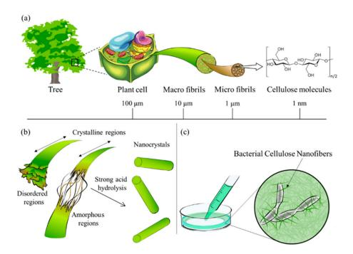
**Figure 4.** (a) Hierarchical structure from the meter to the nanometer scale (cellulose nanofibers) of a natural fiber contained in the plant cell wall; (b) schematic diagram of the isolation of cellulose nanocrystals by strong acid hydrolysis and (c) bottom-up production of bacterial cellulose [68].
