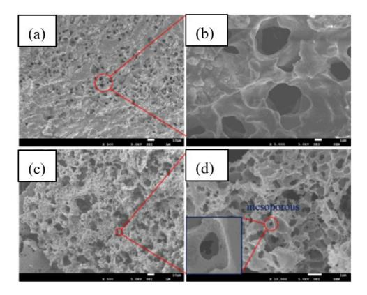
**Figure 17.** Different morphologies of freeze-dried lignosulfonate/ $\kappa$ -carrageenan (**a**,**b**) and their carbon counterparts (**c**,**d**) [264]. Reprinted from International Journal of Biological Macromolecules, 148, Lv, D.; Li, Y.; Wang, L., Carbon aerogels derived from sodium lignin sulfonate embedded in carrageenan skeleton for methylene-blue removal, 979–987, Copyright 2020, with permission from Elsevier.
