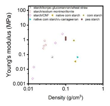
**Figure 31.** Compressive modulus of various porous starches and starch composites: dried with supercritical CO<sub>2</sub> (filled points) and freeze dried (open points) [36,366,370–373].
