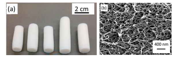
**Figure 18.** κ-carrageenan aerogels prepared via gelation with KSCN: (**a**) monoliths made from solutions of polymer concentration (from left to right) 1; 1.5; 2; 2.5 and 3 wt%, (**b**) scanning electron microscopy image of the fractured surface of aerogel made from 1 wt% solution (adapted from [257]).
