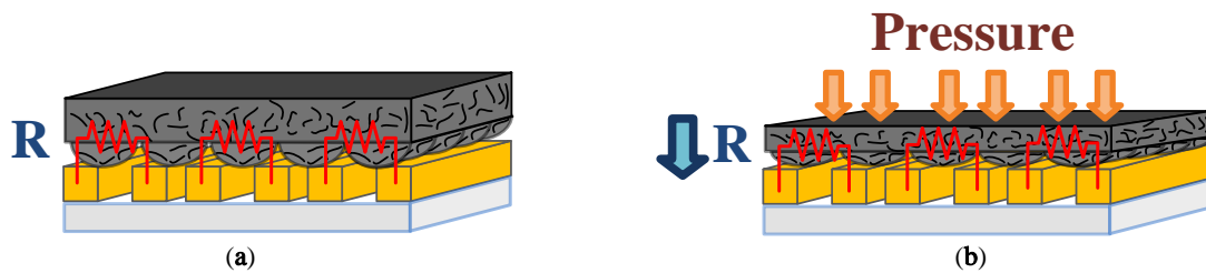
Figure 2. Working principle of the proposed device. (a) The initial shape of the conductive polymer. (b) The microdome structures deform as external pressure is applied.
