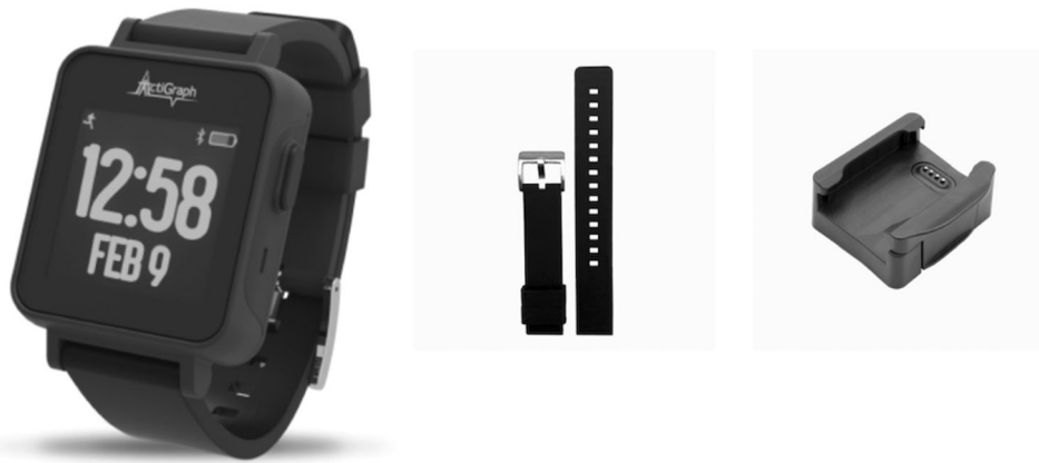
FIGURE 1 ActiGraph CentrePoint Insight Watch (CPIW). The ActiGraph CPIW will be worn as a wristwatch on the nondominant wrist (when identifiable). Commercially available wrist straps adjust the size for small infants and children. The device is easily charged via the wireless charging dock (shown on the right).
