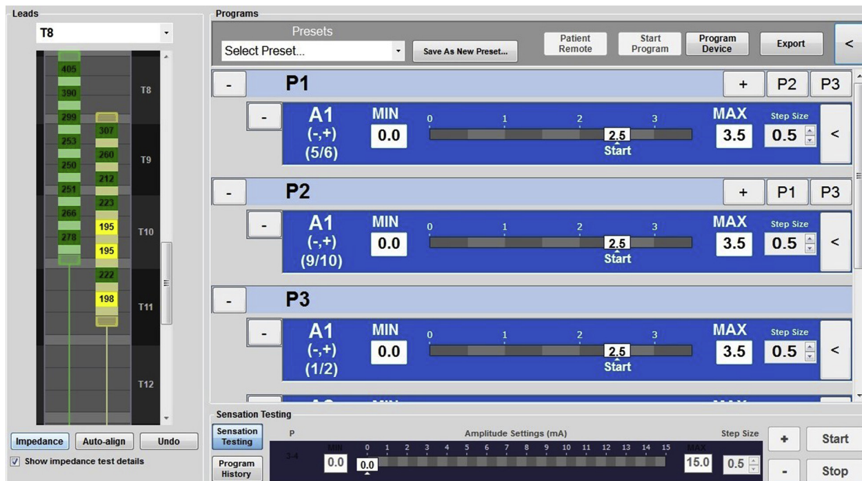
Fig 4. User's interface of the programming software for adjustment, configuration, and impedance measurement of the external or implantable pulse generator.
