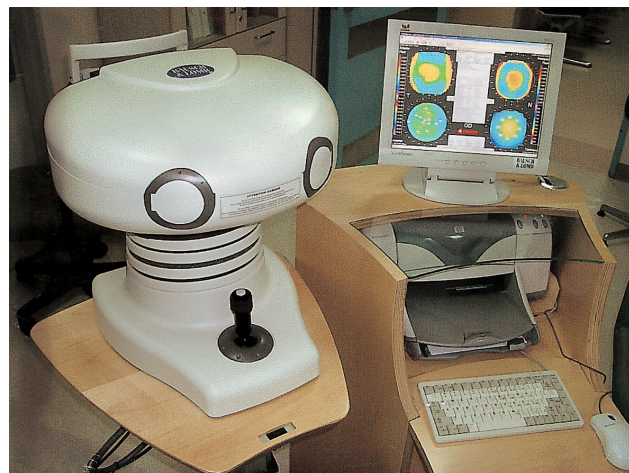
Fig. 2. Orbscan IIz corneal topography system. (Bausch & Lomb, USA)
