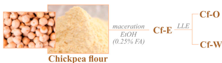
Figure 1. Extraction and fractionation scheme applied to chickpeas before UHPLC-HRMS analysis (FA = formic acid; LLE = liquid/liquid extraction).
