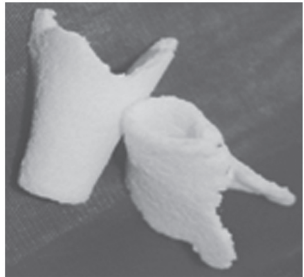
Figure 1. Hollow, semi-flared, porous poly(3-hydroxybutyrate-co-3-hydroxyhexanoate) biomaterials.
