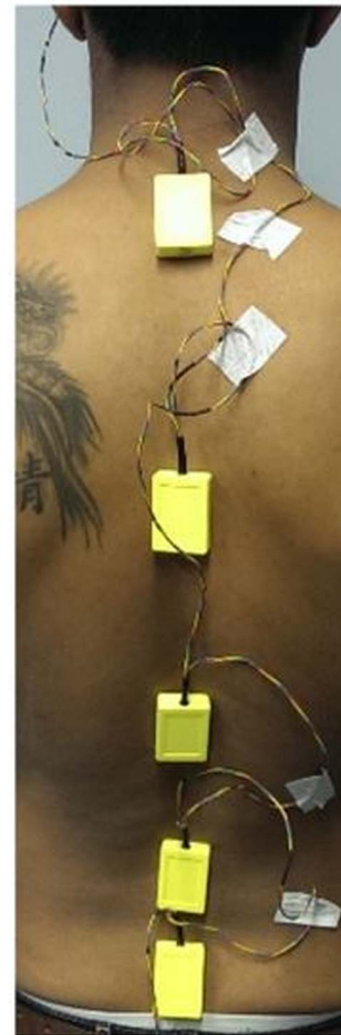
Figure 1 Inertial sensor placements over the spinous processes of C7, T7, T12, L3 and S1.
