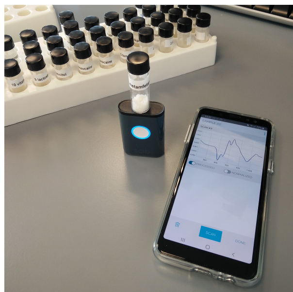
FIGURE 1 Scanning procedure for SCiO near-infrared sensor with the glass sample vial placed directly on top of the light source and detection window [Colour figure can be viewed at wileyonlinelibrary.com ]
