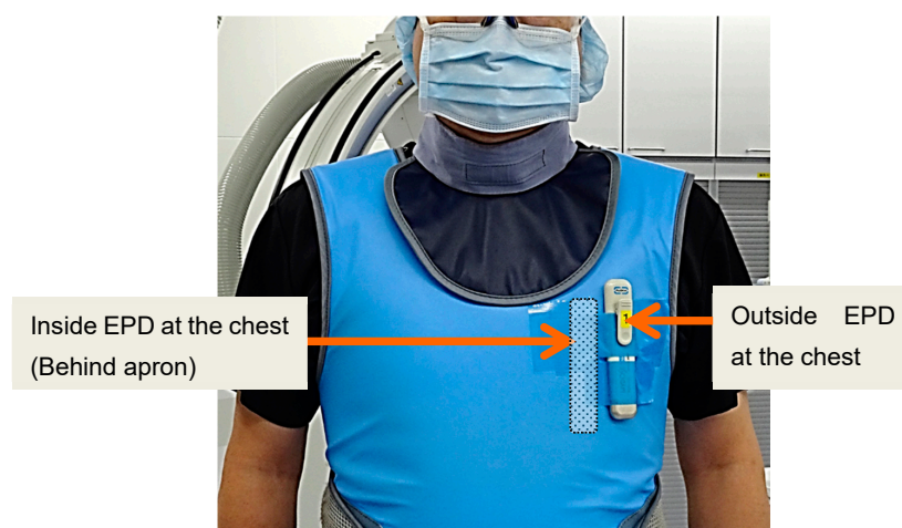
Figure 1. The position of the two electric personal dosimeters (EPDs) worn on the physician's protective apron in a clinical setting.
