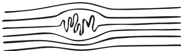
Figure 3. Sketch of the molecular structure assumed in this paper for aligned polyethylene. Most of the material is assumed to consist of parallel molecules with around 5% amorphous regions.
