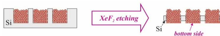
Figure 15. Schematic illustration of the etching in \text{XeF}_2 gas phase applied to remove the silicon substrate surrounding the NdFeB-based micromagnets and to expose their bottom side.
