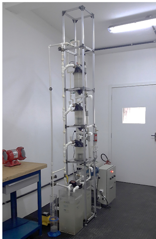
Fig. 3. Bench-scale induced pre-saturation tower with different stages – Patent: BR 20 2017 016076 4.
