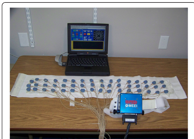
Figure 1 Multidirectional vibrotactile feedback system.
