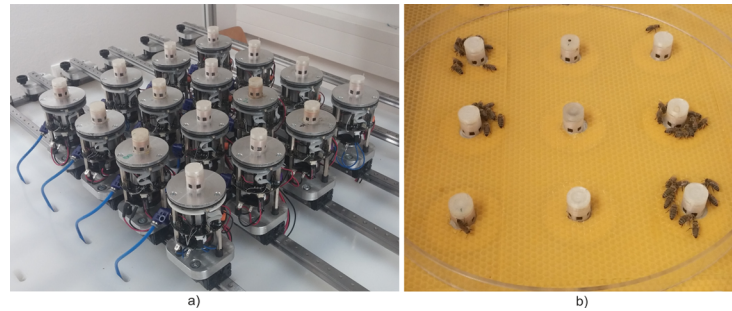
Fig 1. The developed experimental setup. (a) A network of 16 static CASUs without arena floor. (b) The interactive arena with honeybees.
