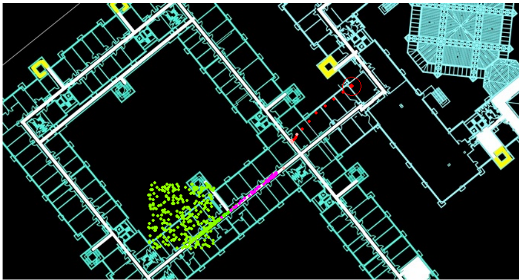
Figure 20. Negative effect of using geolocation service: The red double circle marks the true location while all the particles (marked as green dots) are located far away due to low accuracy geolocation service signals.
