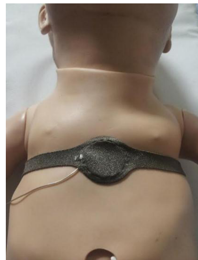
FIGURE 1. The placement of the FingerTPS™ palm sensor on the manikin's chest.
