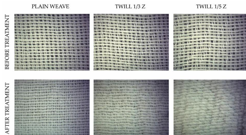
Figure 4. Pictures of samples produced with untreated Co/PBT yarn in weft, before and after thermal treatment of fabrics.
