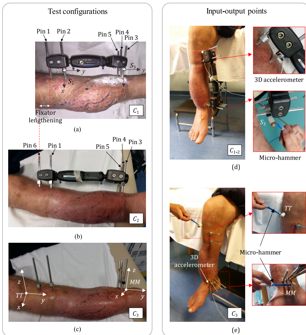
FIGURE 1. Test configurations C_{1-3} (a-c) and test set-up for C_{1,2} (d) and C_3 (e).
