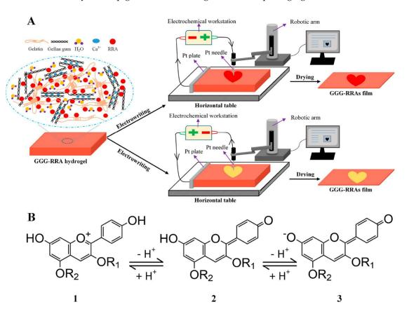
**Figure 4.** (**A**) Principle of electrochemical writing on pH-sensitive films. (**B**) The structure transformation of red radish anthocyanins in acidic and basic conditions. Source: reprinted with permission from Zhai et al. [150], 2018, ACS.
