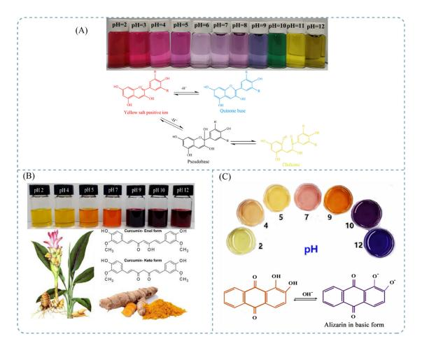
**Figure 2.** Color changes and mechanisms for: (**A**) anthocyanins [5]; (**B**) curcumin [76]; (**C**) alizarin at different pH values [77]. Source: reprinted with permission from Liu et al. [5], 2021, Elsevier; Ezati et al. [76], 2020, Elsevier; and Roy et al. [77], 2021, ACS.
