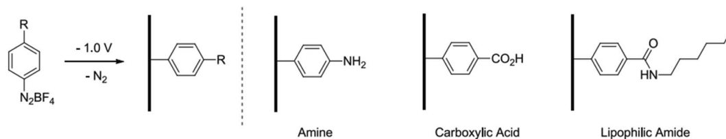
Fig. 2 Schematic of the reductive electrografting of diazo salts (left) and functional groups. 10
