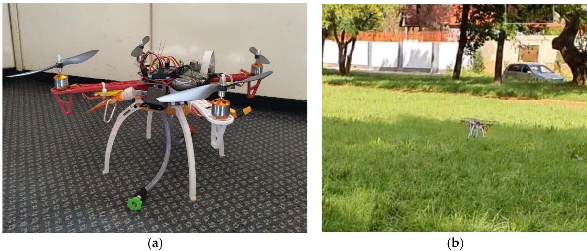
Figure 13. (a) Quadcopter with the sprayer module incorporated; (b) Test-running the smartweed detector and selective herbicide sprayer.
