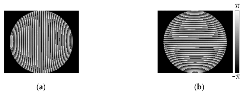
Figure 12. Wrapped phase. (a) Wrapped phase of distorted longitudinal fringe-pattern; (b) Wrapped phase of distorted transverse fringe-pattern transverse.
