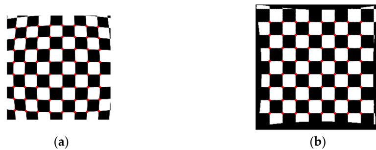
Figure 7. Analyzed results of checkerboard image, where the red points represent the corners. (a) Distorted checkerboard image with distortion parameter \lambda = -1 \times 10^{-6} and distortion center (289, 273); (b) Corrected image.
