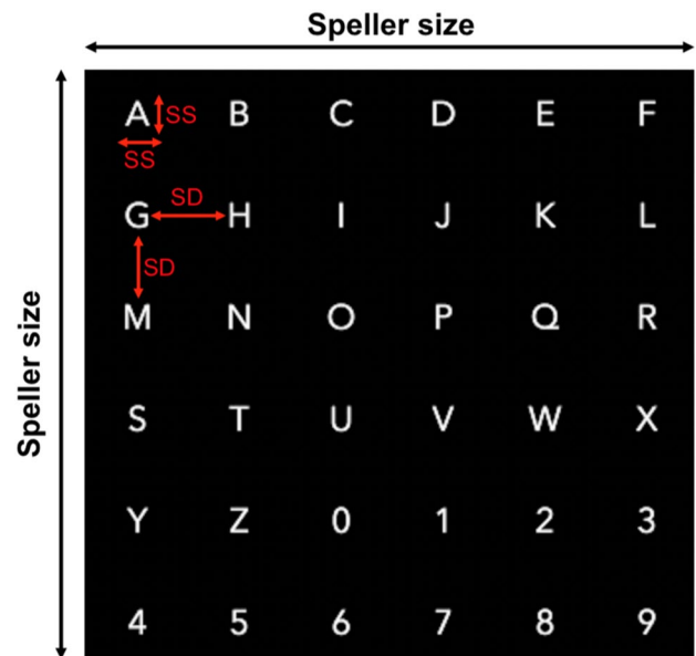
Fig. 5 Example of speller’s size parameters. SS stands for “symbol size” and SD for “symbol distance”
