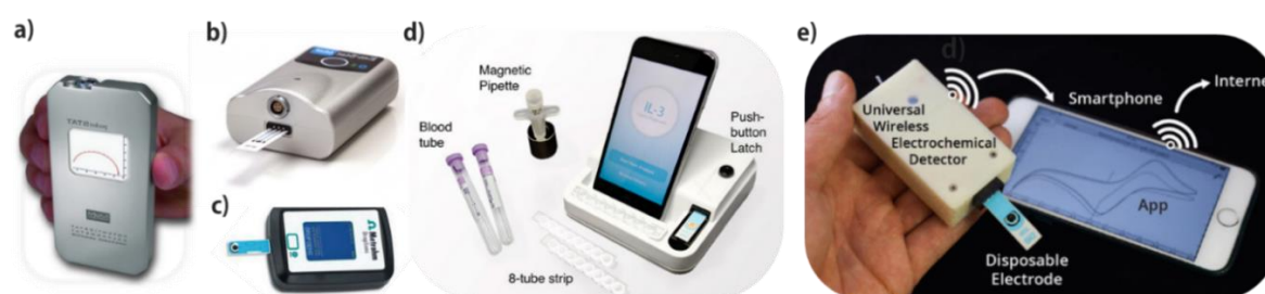
Figure 1. Examples of hand-held electrochemical readers as (a) PocketStat (IVIUM Technologies®), (b) EmStat (PalmSens®) and (c) DropStat (DropSens®); (d) integrated biosensor for Sepsis diagnosis (adapted from reference [13] with permission of American Chemical Society); and, (e) universal wireless electrochemical detector (UWED). Reproduced with permission from [14].
