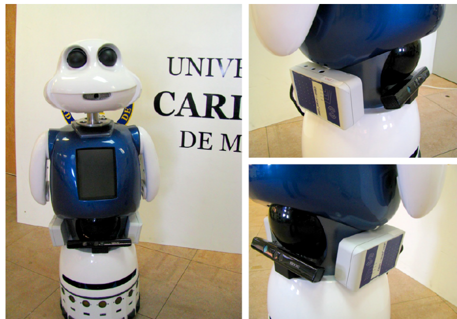
Figure 1. The social robot Maggie and its two RFID UHF readers/writers.
