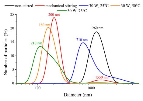
**Figure 3.** Number-based size distribution curves of the nickel nanoparticles prepared without stirring (25 °C), with mechanical stirring (25 °C) and under ultrasonic treatment (30 W output power, continuous sonication) at various temperatures.
