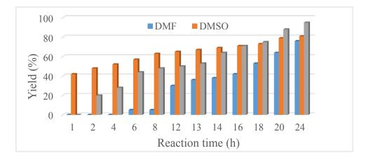
**Figure 6.** The biphenyl yield in the reaction of iodobenzene and phenylboronic acid in different solvents using Ni catalyst prepared with continuous ultrasound treatment (30 W output power) and at reflux temperature.
