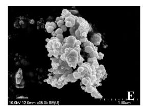
**Figure 5.** Scanning electron microscopy images of the selected NiNPs (**A**: non-stirred, **B**: mechanically stirred, **C**: 30 W - 20%, **D**: 30 W - 100%, **E**: 120 W - 100% ultrasonically treated samples).
