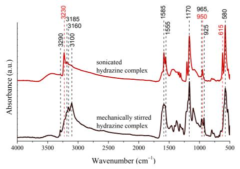
**Figure 2.** Infrared spectra of the nickel-hydrazine-iodide complexes formed on mechanical stirring or sonication (30 W output power and continuous emission) for 4 h at 75 °C.
