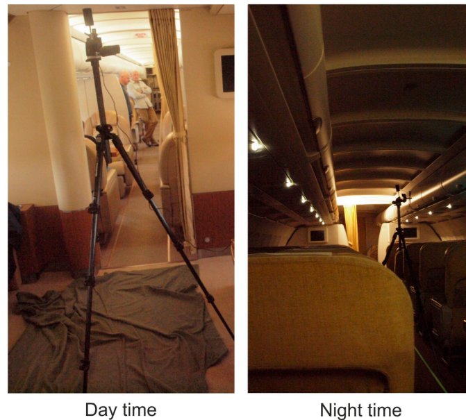
Figure 16. Measurement of illumination parameters to determine ASLODE on board the Airbus A-319CJ.
