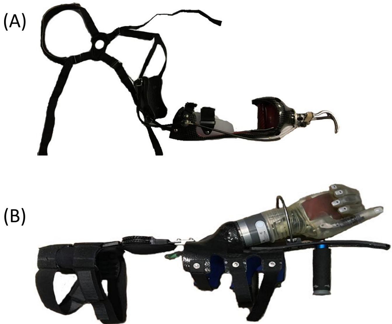
Fig 1. Upper limb prosthesis bypass devices. A) Body Powered Bypass device, right side configuration with body-powered voluntary open Hosmer 5x split hook terminal device. B) DEKA Bypass device, right-hand radial configuration with powered wrist.
