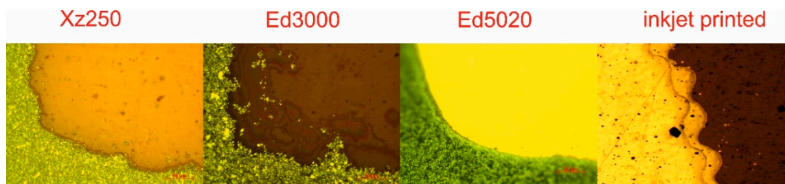
Figure 9. The edges of the realized UWB antenna by screen-printing with the 400 mesh and inkjet-printing technology.
