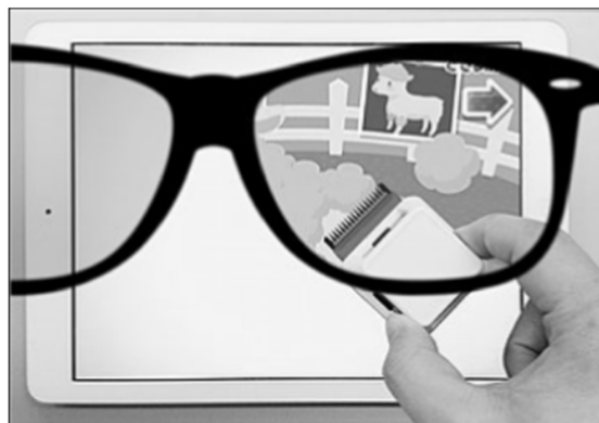
Figure 3. Appearance of the Occlu-pad. Only the right eye can see the image of the tablet terminal, while the left eye cannot.
