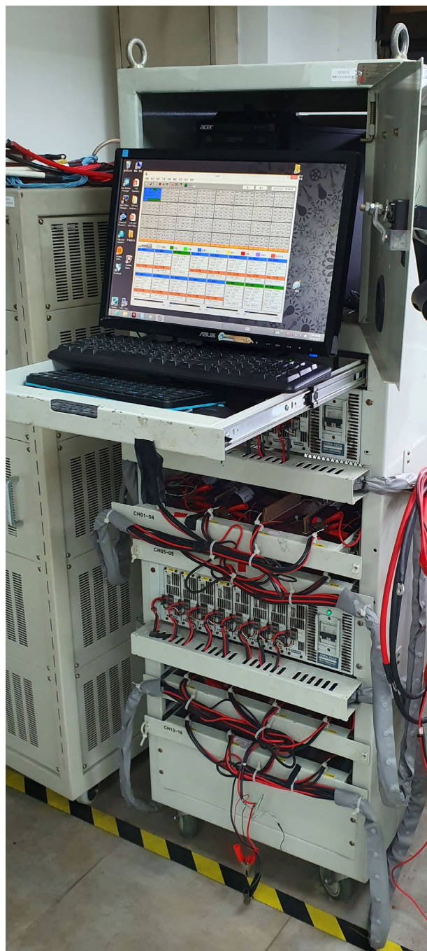
Fig. 3 Battery test system. The CTE-MCP-5082020A battery test system (made by Chen Tech Electric Mfg. Co., Ltd., Taiwan) is used for evaluating the performance of the battery cells. There are 16 channels, and each of them can provide measurements of voltage, current, and temperature simultaneously.
